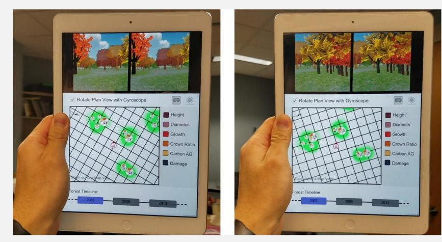
As the 3D view is rotated, the linked 2D view rotates correspondingly.
